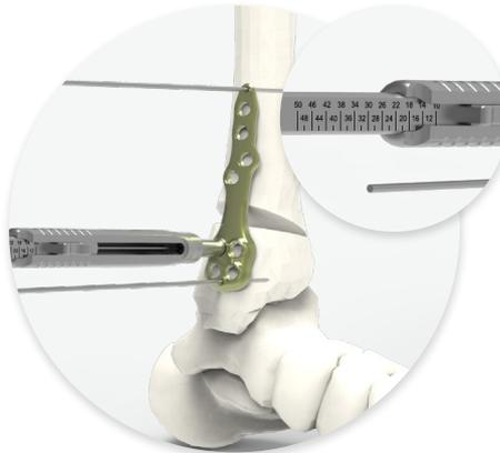
5. Depending on the type of drilling used (see steps 4a and 4b), determine the drilling depth directly on the threaded guide gauge (ANC1094) or with the length gauge (ANC1095).
