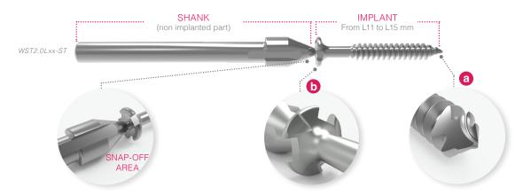
**Snap-off screw :** the screw separates itself from the shank as soon as the head gets in contact with the bone. **N.B:** For an additional compression, use the screwdriver (ANC770).
