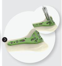
8. In order to support the distal part, proceed in the same way as steps 5 and 6 for the monoaxial hole in the window.
