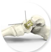
Position the plate on the medial side of the talo-navicular joint and insert two Ø1.2 mm pins (33.0212.070) in the navicular part.
